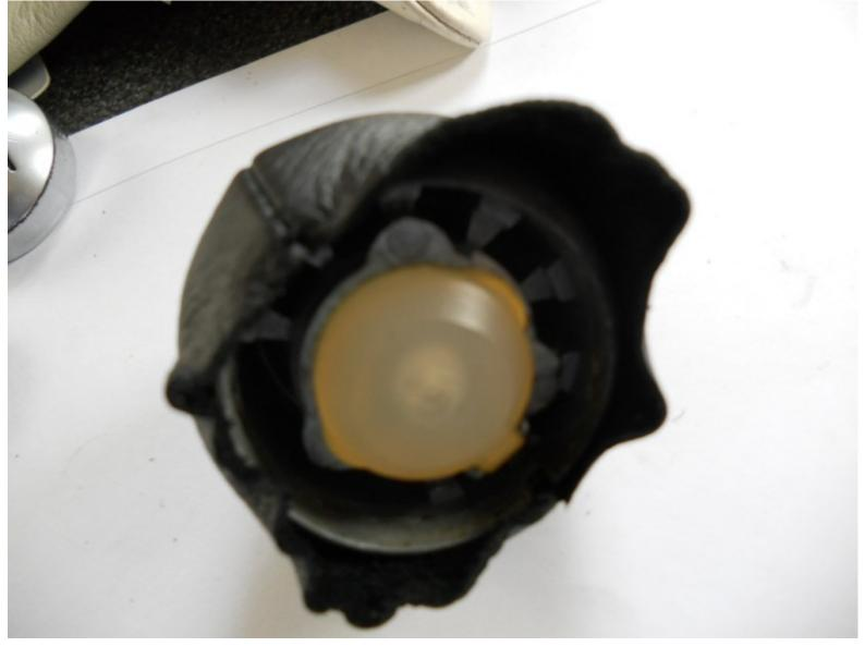
9. Replace the black plastic ring and the silver part. There will be "guides" (two double prongs see above) on the plastic top to ensure it goes in the "right way up" for when you put it back in the car. This may need a bit of force, I eventually used a small rubber camping mallet so as not to break the plastic. Both parts tighten the new leather cover so the "grain" is stretched to leave the knob fairly smooth and looking like new...if slightly out of focus.
