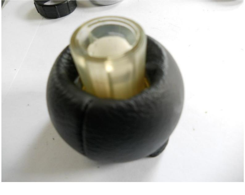
3.Remove black plastic ring from bottom. Finger tight, perhaps lever with small screwdriver.
