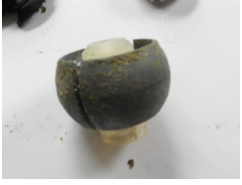
7. The new cover looks like this, Ease it over the cleaned metal knob. Slide it over the metal knob with the seams lined up with the channels.
