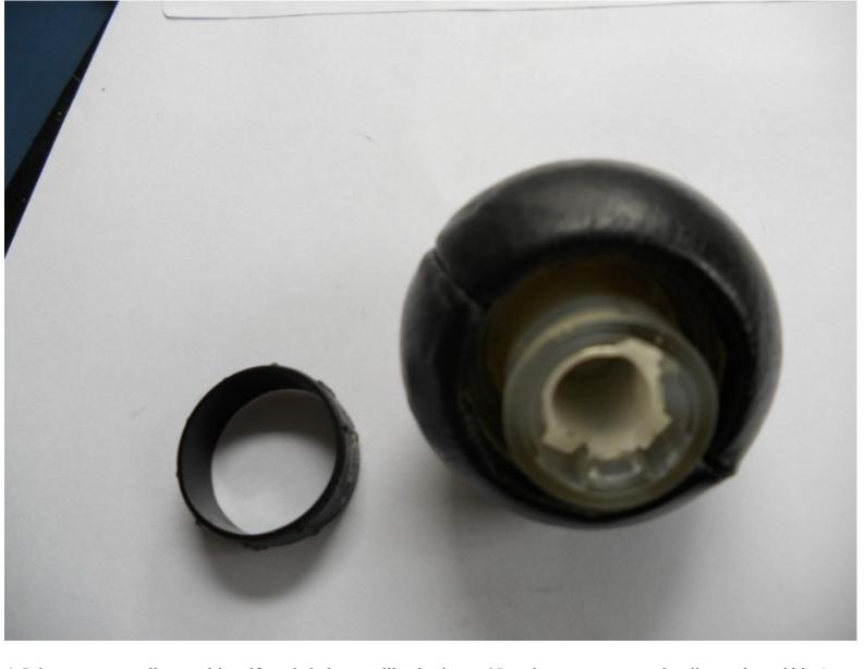
4. Prise out, use small screwdriver if needed, the metallic plastic top. Note the two prongs on the silver coloured bit. (sorry slightly out of sequence).
